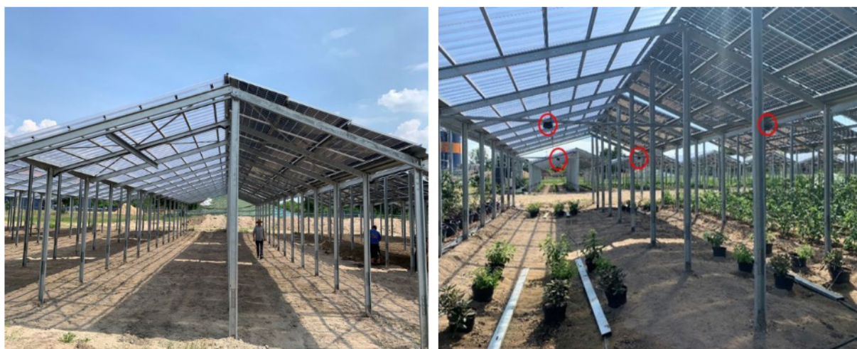
Figure 3. SUNfarming Food & Energy system (left) and experimental setup (right). Positions of the cameras used for monitoring plant growth under the panel and the acrylic glass section of the system marked with red circles. Plants were grown for 12 weeks after being transferred from the nursery to Rathenow.
